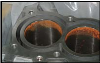
Standard Corrosion Protection Packaging: RUSTED
