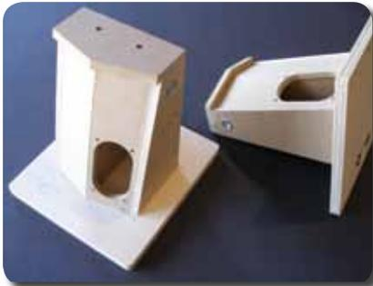
Packnet also provided precision waterjet cutting services of felt and water resistant dense chipboard for the chair
