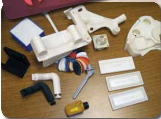
Some examples of parts that have been created include components of a lawn mower, moving pulley parts, threaded inserts, display panels as well as various tools such as a crescent wrench.
